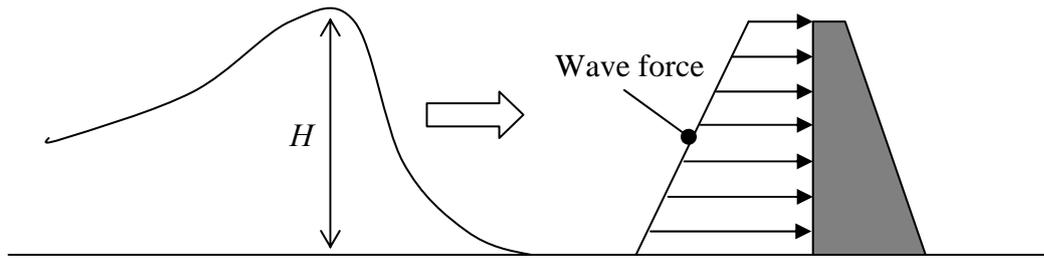
Figure 7 Lateral wave force distribution acting on a seawall
