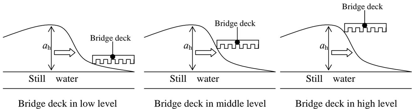
Figure 8 Experiment on wave force acting on a bridge deck in 3 different levels
