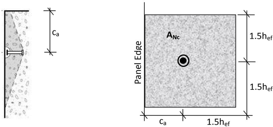
**Fig 5: Idealised single edge truncated failure cone**
