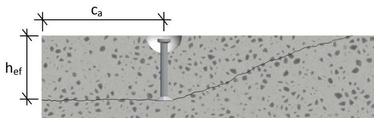
**Fig 13: Idealised fracture path as stated in ACI318M-08 for a single cast-in anchor**
