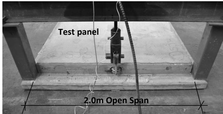
**Fig 11: Shear loads applied with 2.0m open span reaction frame**
