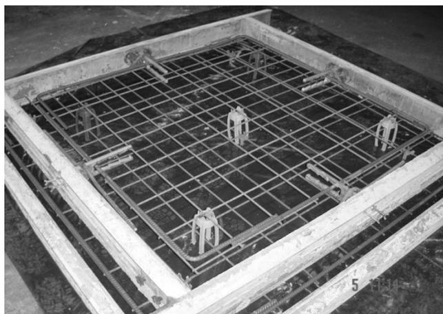
**Fig 4: Typical shear panel setup prior to concrete pour**
