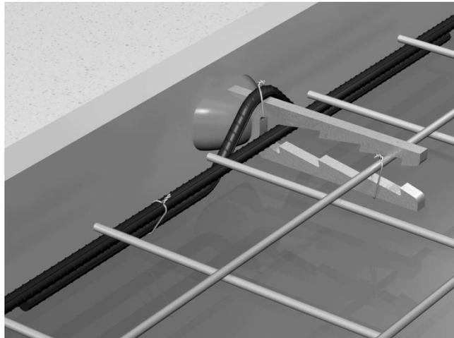
**Fig 3: View of a typical anchor setup for thin panel edgelifting**
