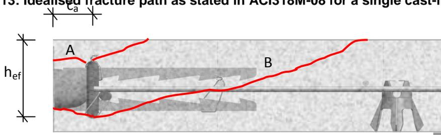
**Fig 14: Estimate fracture path from test results**
