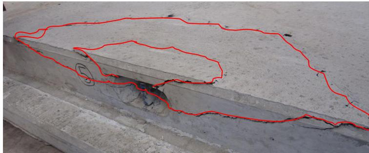
**Fig 15: Actual fracture surface**
