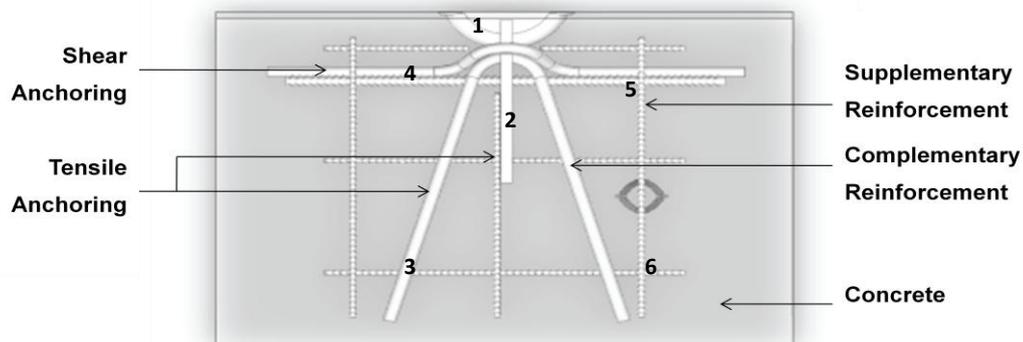
Fig 1: Plan view of a typical panel setup for edgelifting
