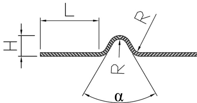
**Fig 6: Typical shear bar design**
