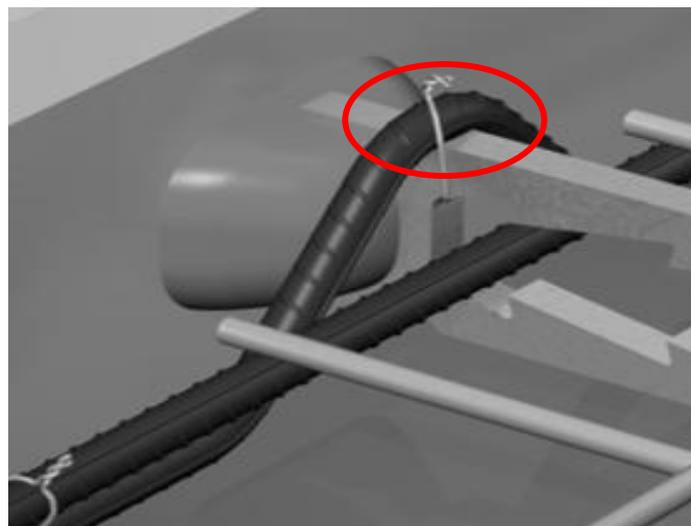
**Fig 7: The shear bar bridge is subjected to bending when a shear load is applied**
