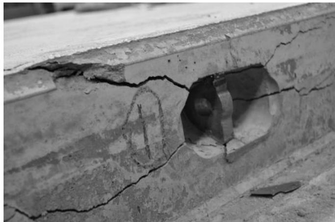
**Fig 12: Typical failure surface propagating to the panel thin edge**
