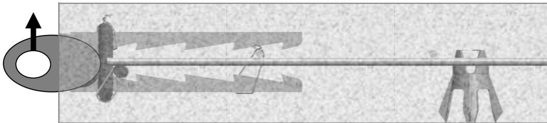
**Fig 8: Shear loads applied in a lateral tensile direction**
