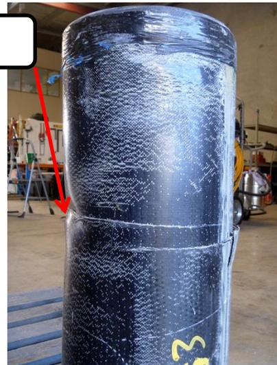
Figure 6. Failure of NS-J-2
