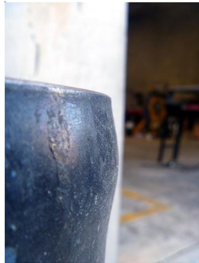
Figure 4. Failure of NS-C-1 (Detail)
