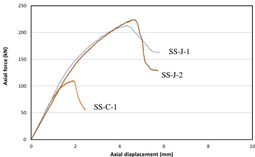
Figure 10. Axial load and displacement response – SS specimens
