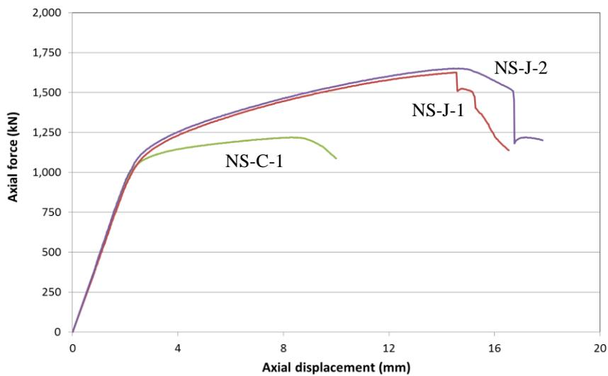
Figure 7. Axial load and displacement response – NS specimens
