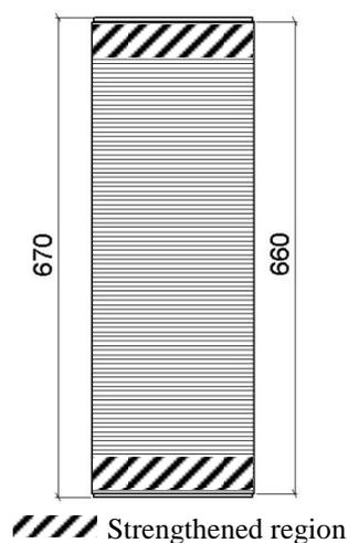
Figure 1. Test specimen
