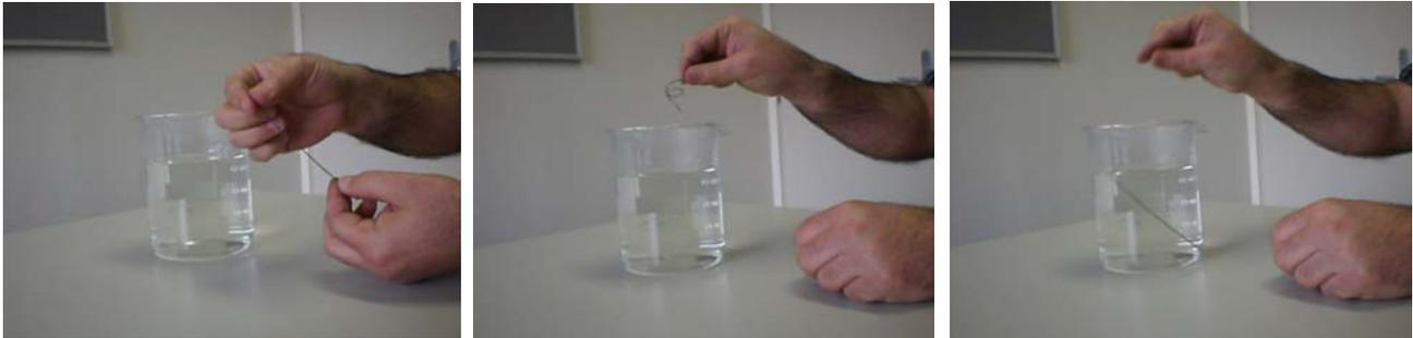
(a) initial shape: straight wire    (b) bent wire dropped in hot water    (c) initial shape recovered
