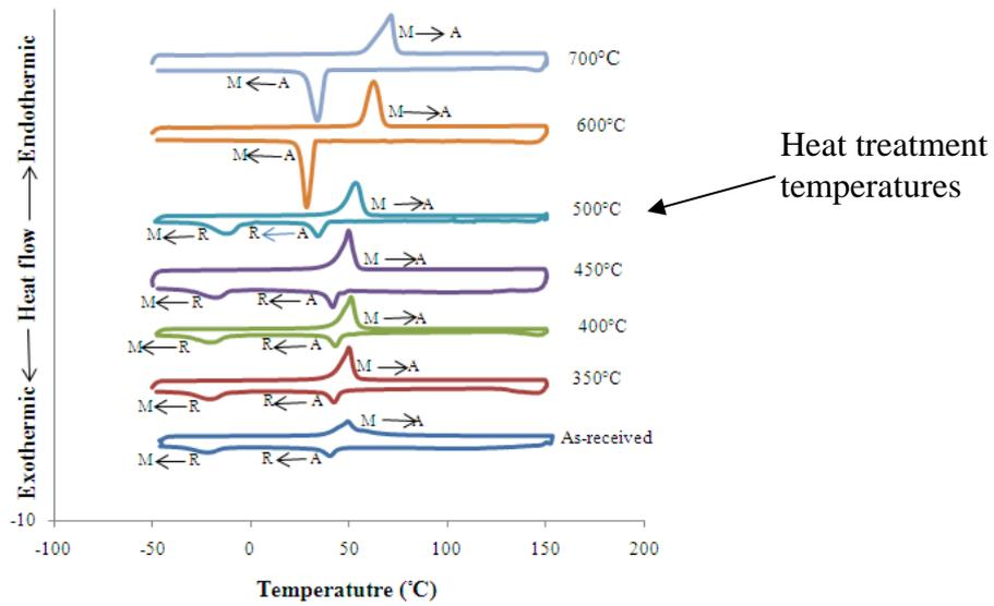
**Figure 3.** Effect of heat treatment temperatures on phase transformation of shape memory alloys (Sadiq, et. al., 2010).
