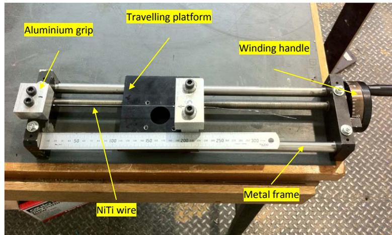
**Figure 7.** Pre-straining equipment for NiTi wires.
