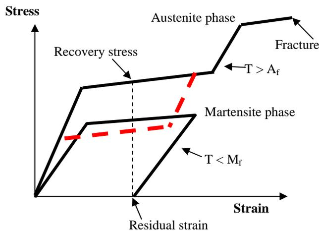
**Figure 4.** Super-elasticity and shape memory effect of SMA.
