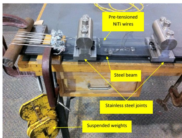
**Figure 6.** Specimen assembly for the high temperature test.
