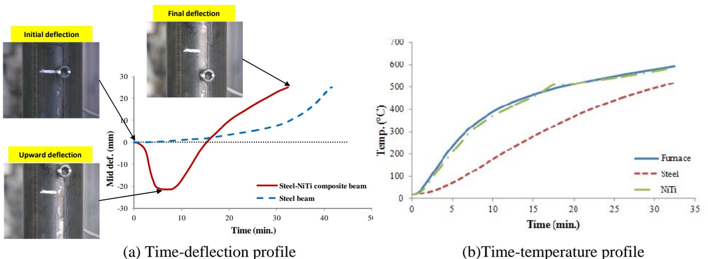
**Figure 9.** Mid-span deflections and temperatures of steel and steel-NiTi composite beams.
