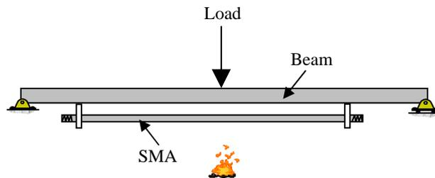
**Figure 5.** Steel beam strengthened by SMA wire in fire.
