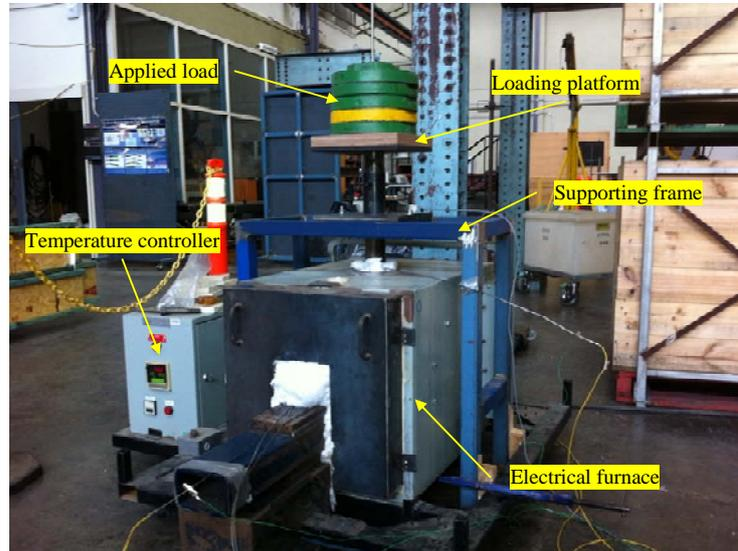
**Figure 8.** High temperature test setup.
