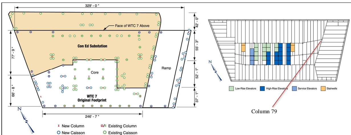
**Figure 8. WTC 7 Foundation Layout and Typical Framing Plan**
