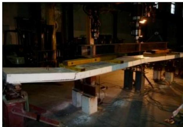
Figure 11. Photograph at failure of slab S3-20-00
