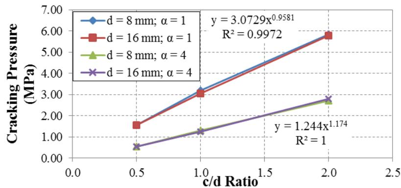
**Figure 10:** Effect of bar diameter, cover depth-to-bar diameter ratio on the cracking pressure of uniform and pitting corrosion
