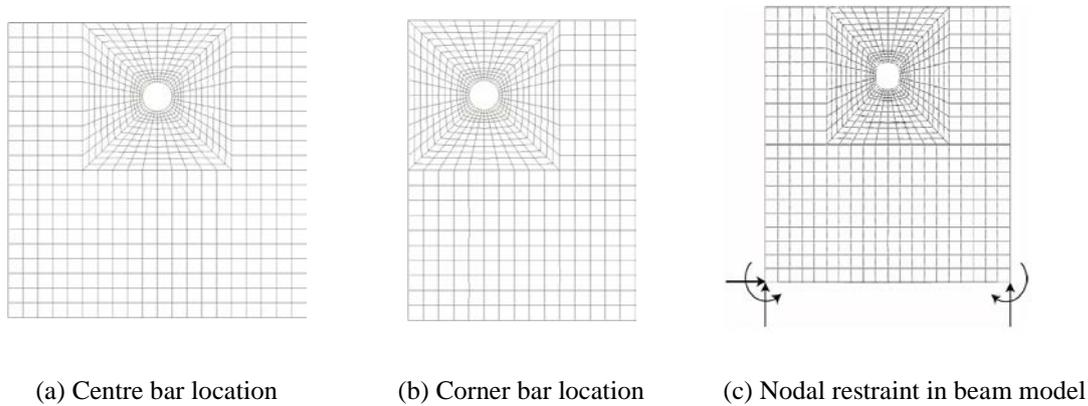
**Figure 2:** Finite element meshes.
