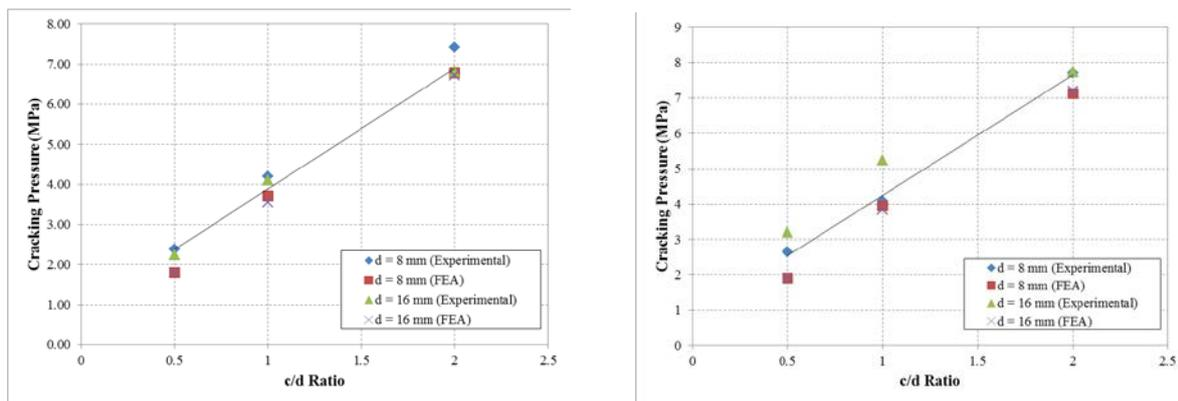
**Figure 11:** Comparison of model result with experimental data (Williamson and Clark, 2000) (Left figure: rebar at the centre and right figure: rebar at the corner)
