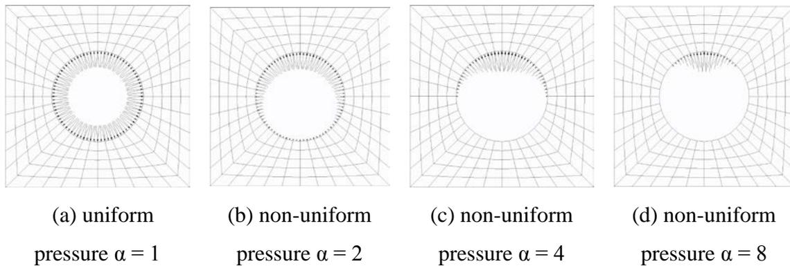
**Figure 3:** Uniform and non-uniform pressure distributions around reinforcement bar (Jang and Oh, 2010).
