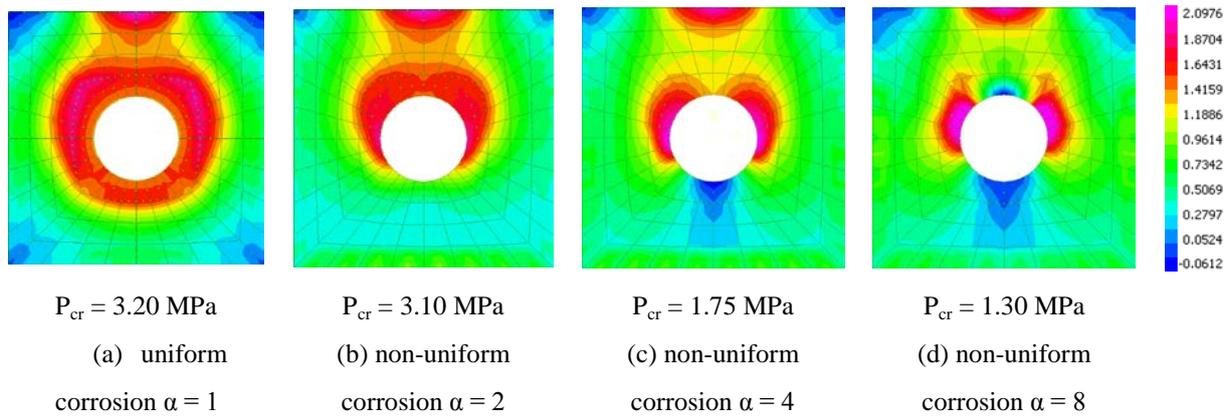
**Figure 5:** Effect of non-uniform corrosion on the cracking pressure ( $P_{cr}$ ).
