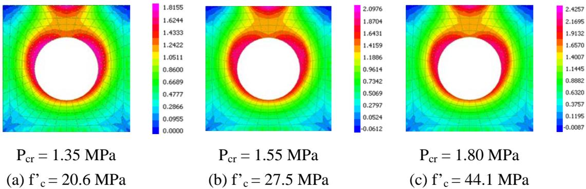
**Figure 7:** Effect of concrete strength on the cracking pressure  $P_{cr}$
