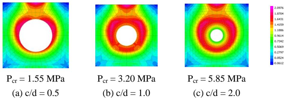
**Figure 9:** Effect of cover depth on the cracking pressure ( $P_{cr}$ )
