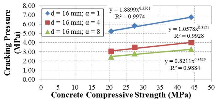
**Figure 8:** Cracking pressure as a function of compressive strength for various  $\alpha$  values
