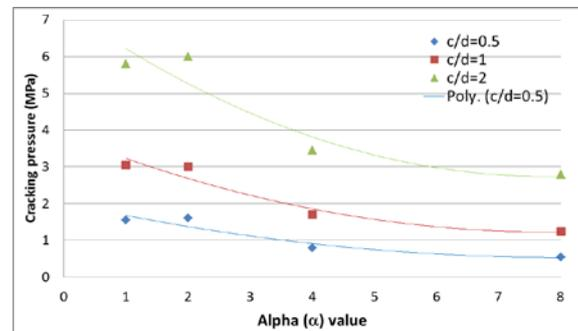
**Figure 6:** Effects of corrosion distribution and concrete cover on the cracking pressure.
