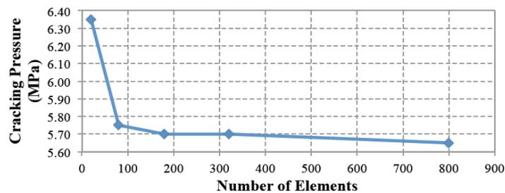
**Figure 4** Effect of number of elements on the cracking pressure
