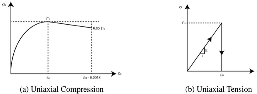
**Figure 1:** Idealised stress-strain curves for concrete.
