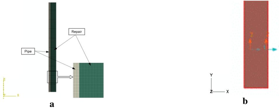
Figure 1: (a) FEA mesh, (b) Material orientation for repair laminate
