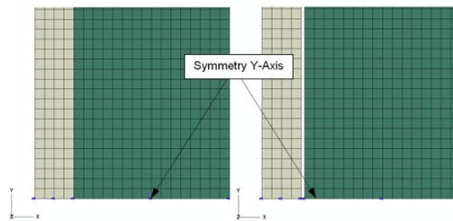
Figure 2: Boundary condition definition for the FEA model
