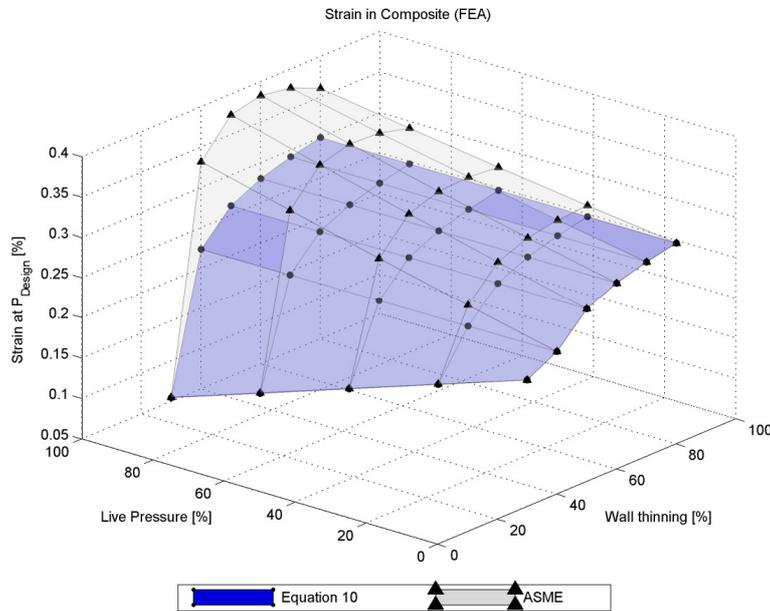
Figure 4: Comparing strain in the Composite at design pressure
