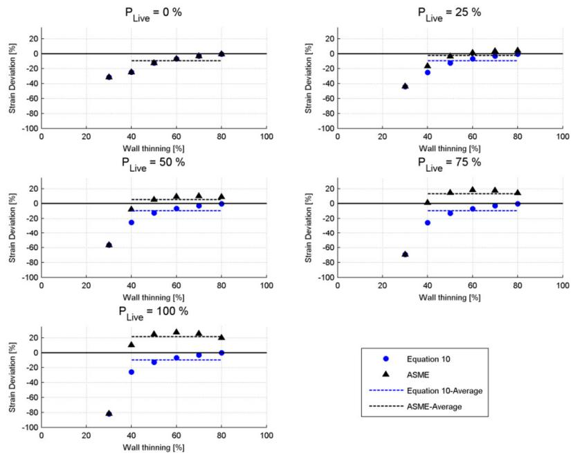
Figure 5: Strain deviation in the composite repair at design pressure
