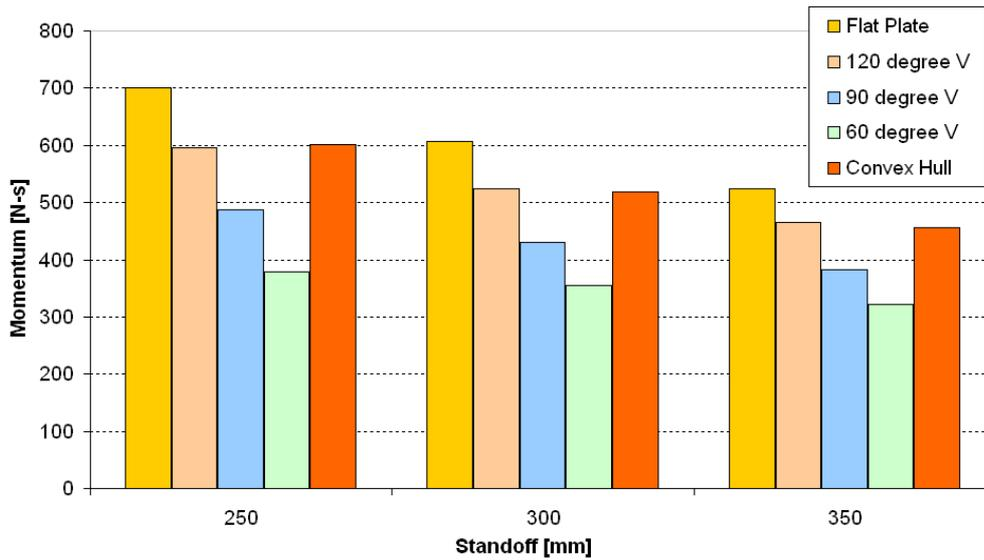
**Figure 4** Comparison between vertical momentum transferred for different hull geometries and standoff distances for charges placed under the centreline of the hull.
