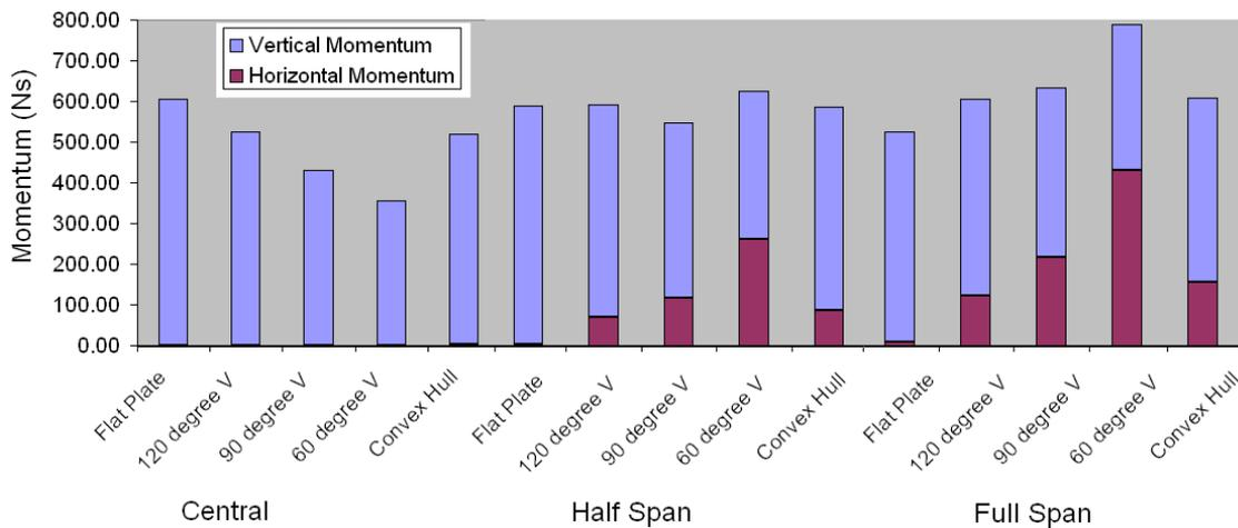
**Figure 8** Breakdown of total momentum transfer to targets for different charge locations.
