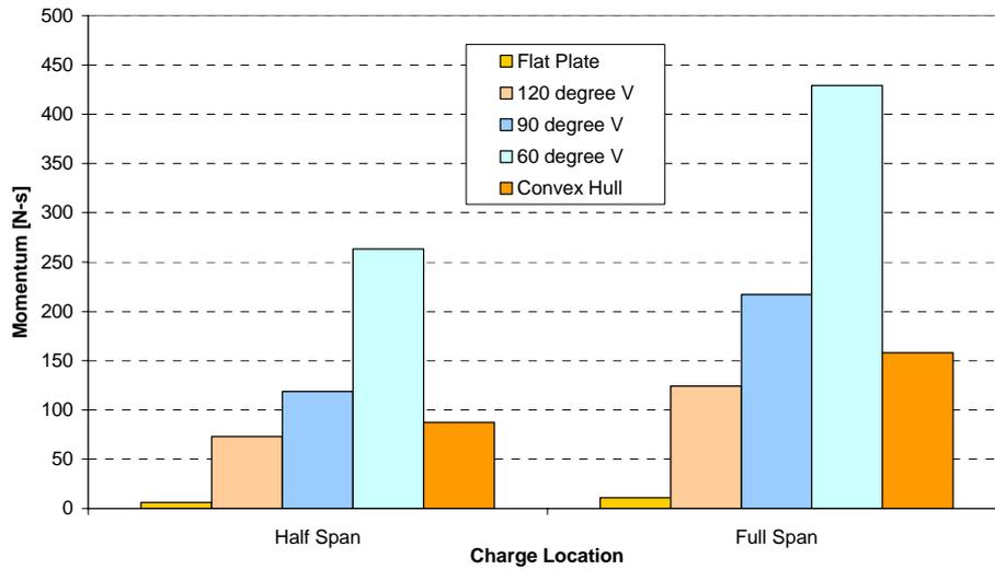
**Figure 7** Comparison between horizontal momentum transferred for different hull geometries at different charge locations.
