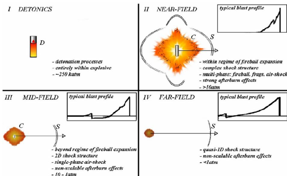
Figure 1 Four regimes of blast wave propagation (Ritzel 2006).
