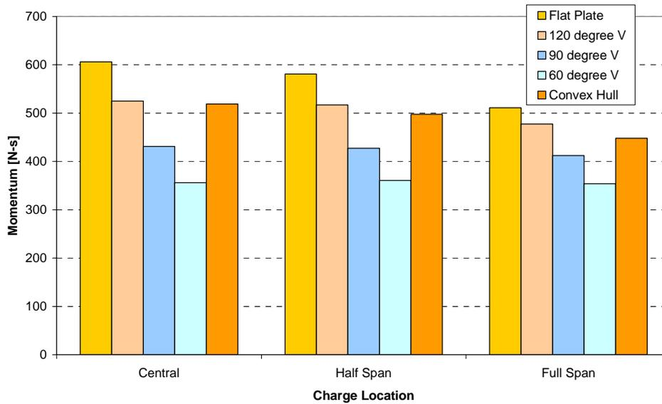
**Figure 6** Comparison between vertical momentum transferred for different hull geometries at different charge locations at a standoff distance of 300 mm.
