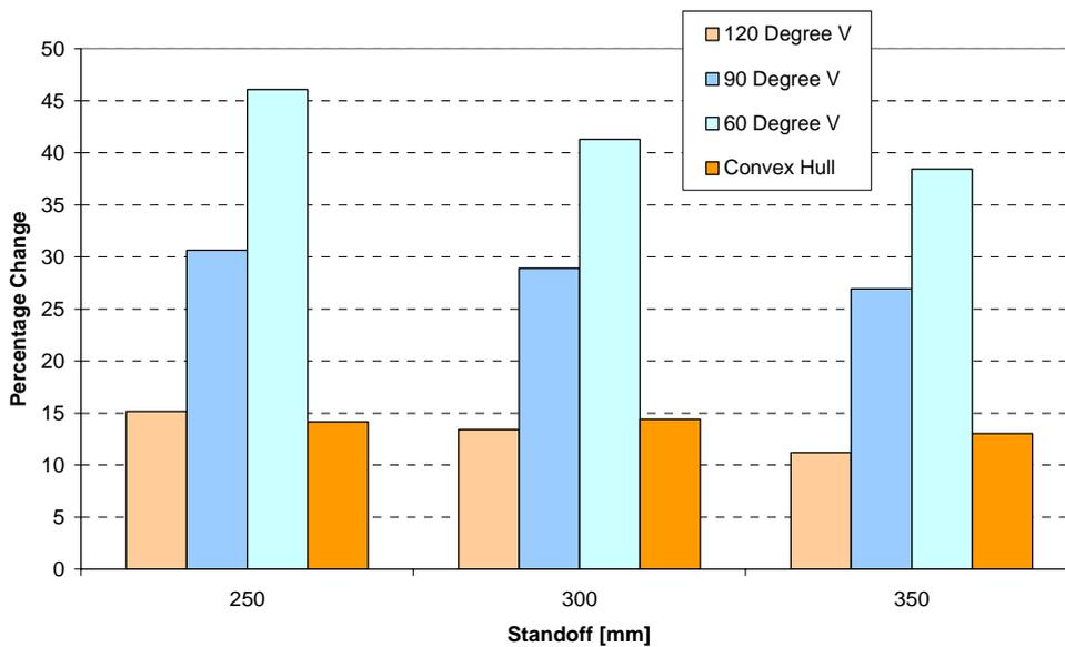
**Figure 5** Percentage reduction in the vertical momentum transferred to different hull geometries when compared to the flat plate at the corresponding standoff distances for charges placed under the centreline of the hull.
