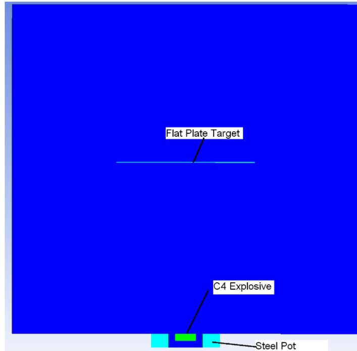
**Figure 2** Arrangement of model with flat plate as target.
