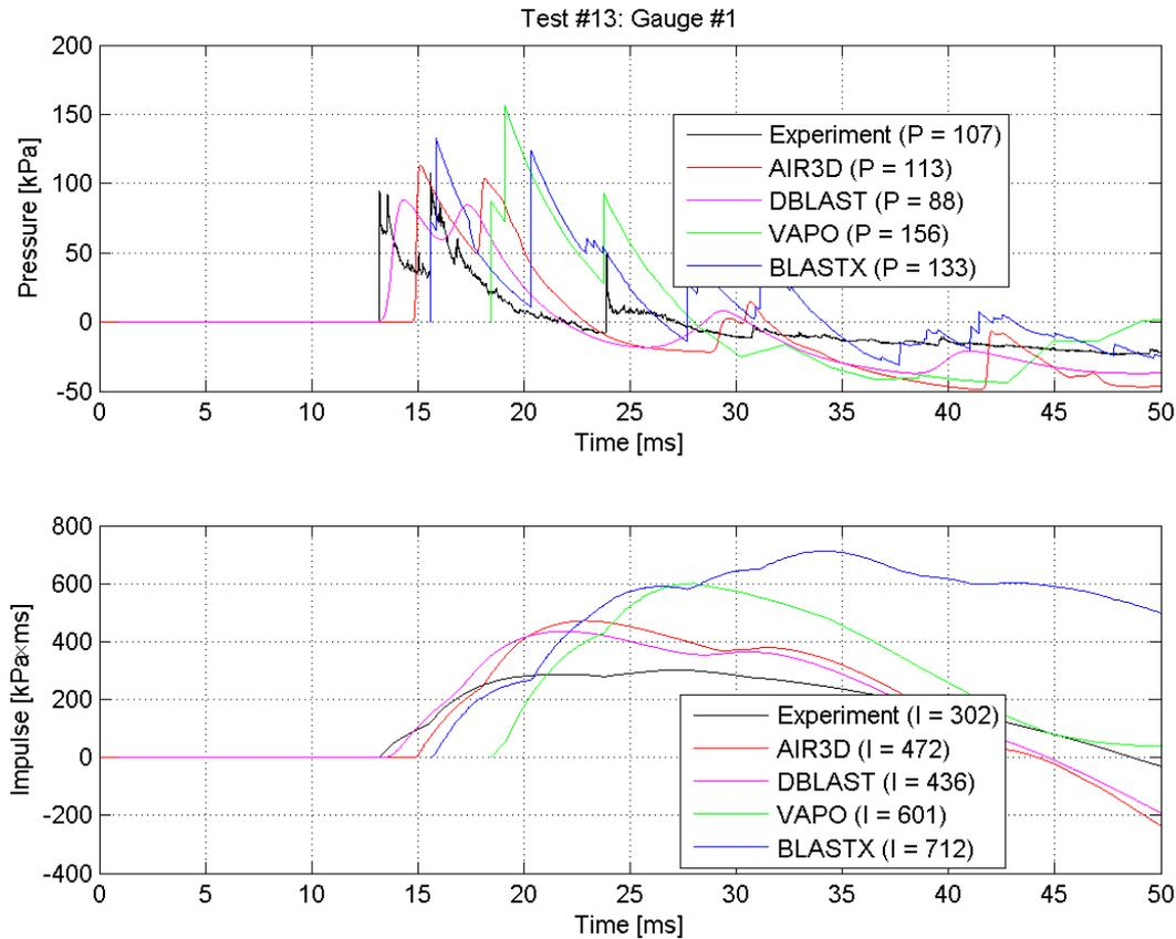
**Figure 5.** Measured and predicted pressure traces at Gauge #1 (Test #13).
