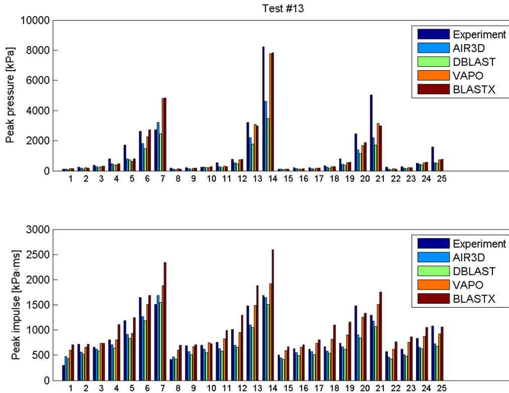
**Figure 3.** Comparison of measured and predicted peak pressure and impulse (pressure gauge numbers shown on x-axis).
