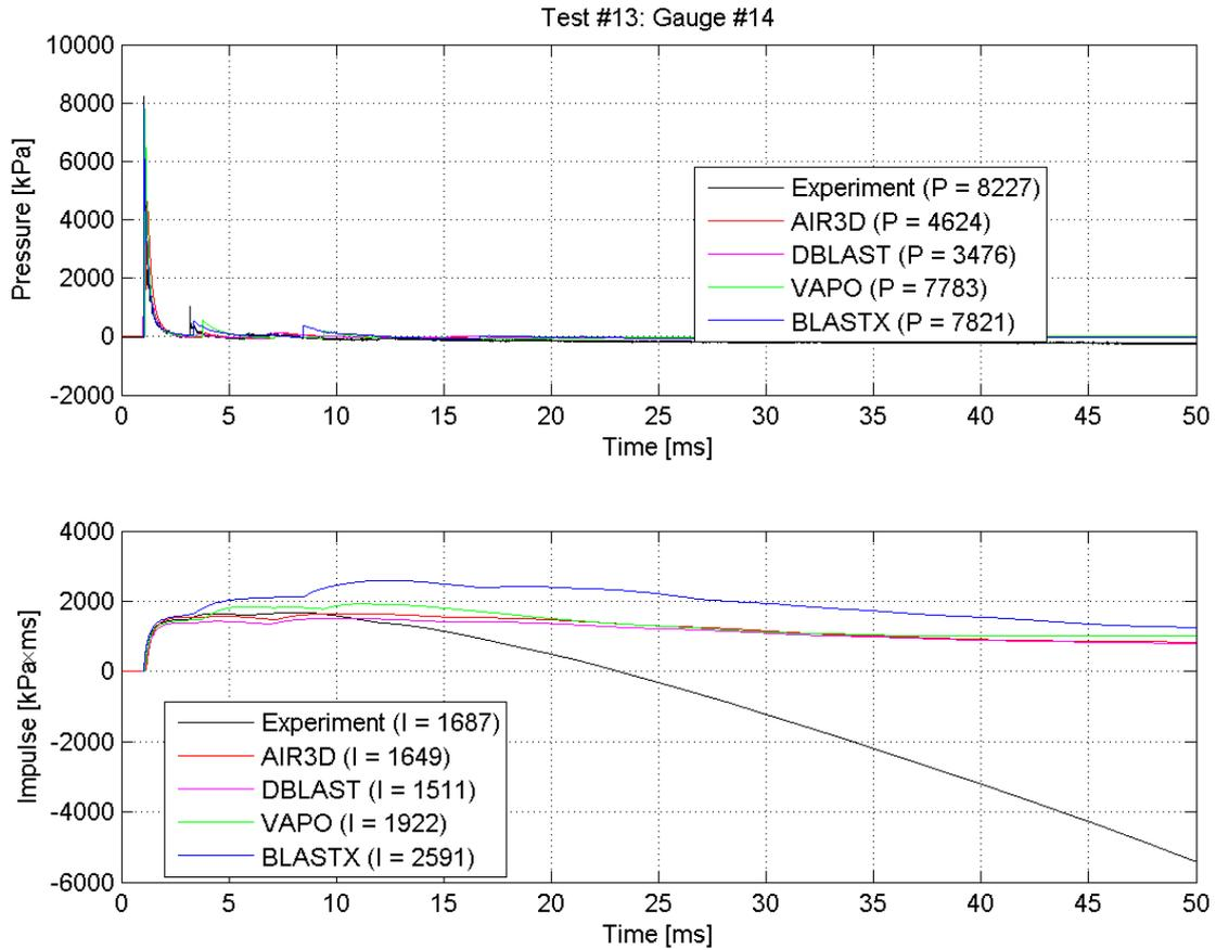
**Figure 4.** Measured and predicted pressure traces at Gauge #14 (Test #13).
