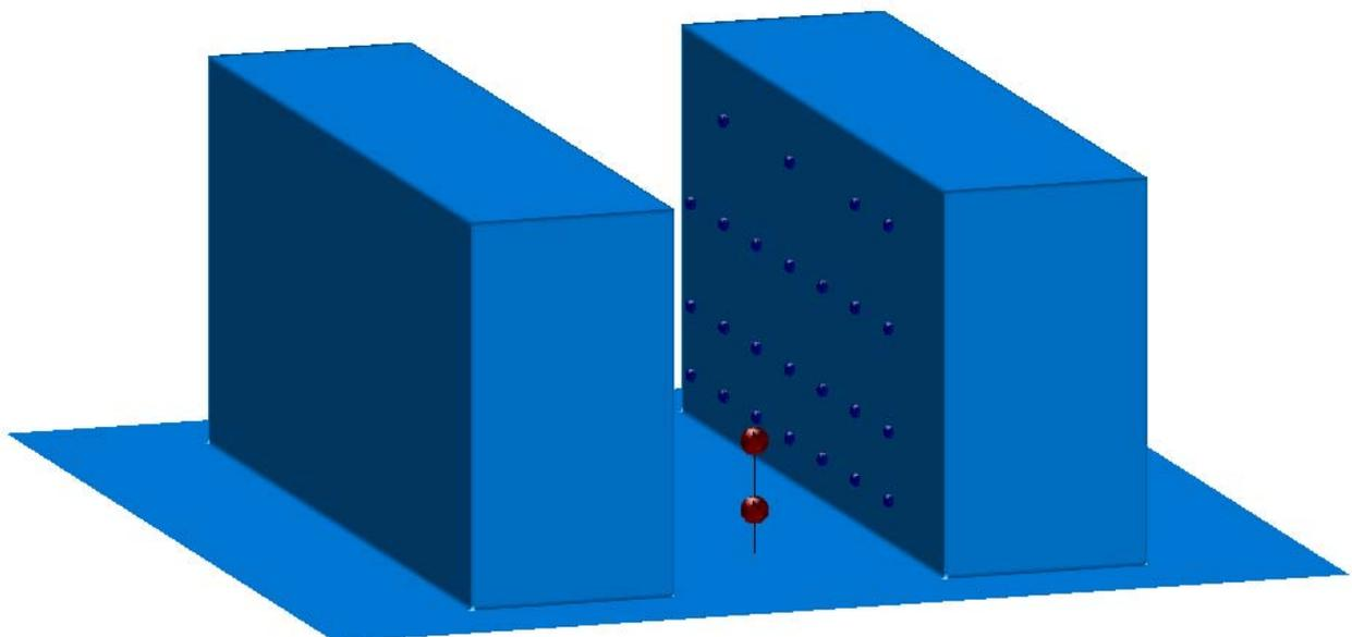
**Figure 2.** Two charge positions and 25 activated pressure gauges.
