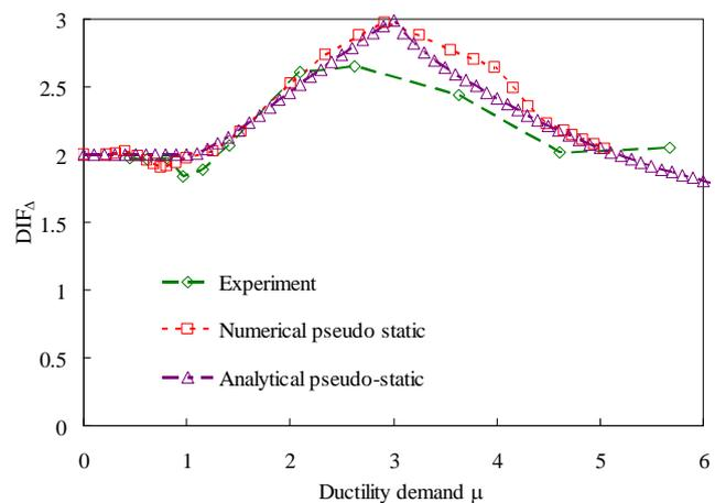
Figure 8 Prediction of displacement-based DIFs
