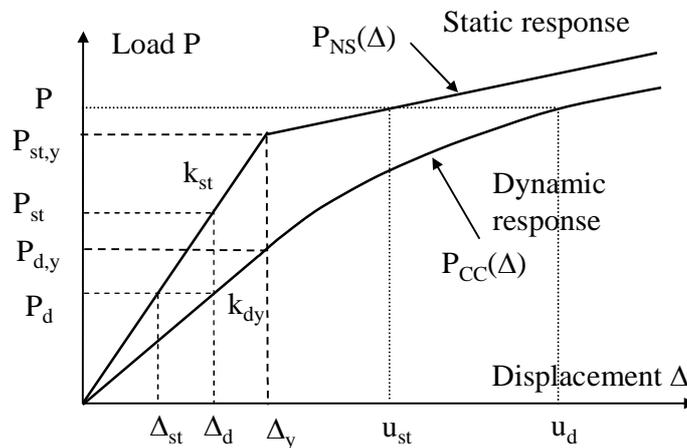
**Figure 5** Explanation of the definition of displacement- and force-based DIFs
