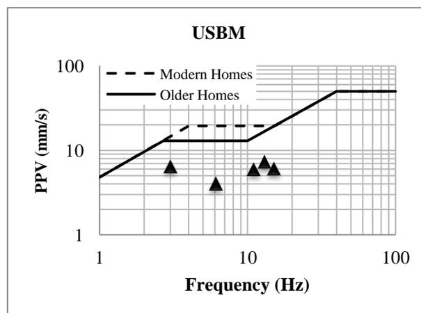
**Figure 4.** Evaluation of damage risk according to USBM criteria
