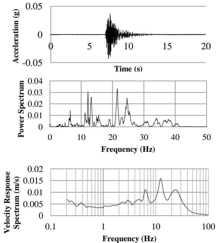
**Figure 1.** Recorded horizontal ground acceleration, its response spectrum and power spectrum.
