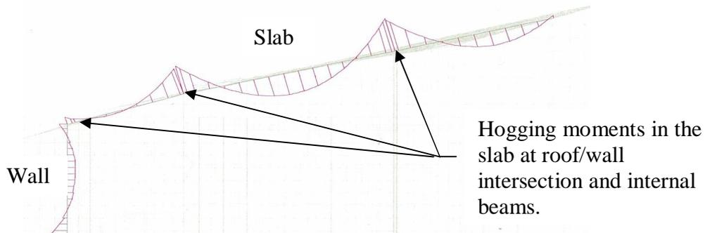
**Figure 10.** Typical bending moment diagram output by Microstran
