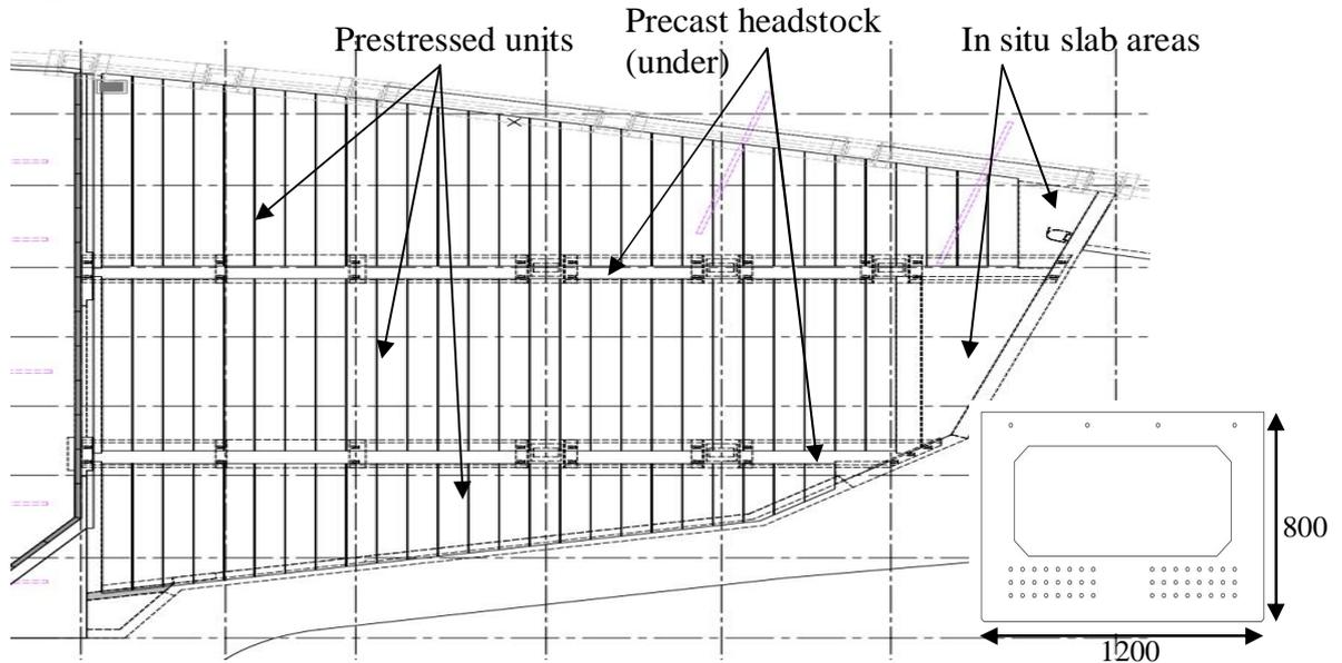
**Figure 8.** Roof plan and a cross-section of a typical prestressed unit
