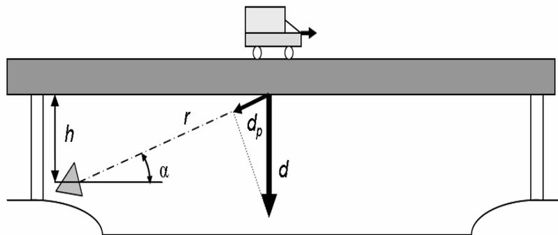
**Figure 4:** Example of Resolving Measured Movement as a Deflection (Lee 2010)
