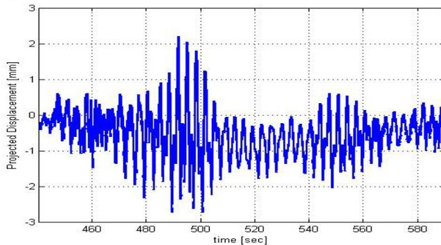
**Figure 5:** Time domain data collected during testing of the Soul Building
