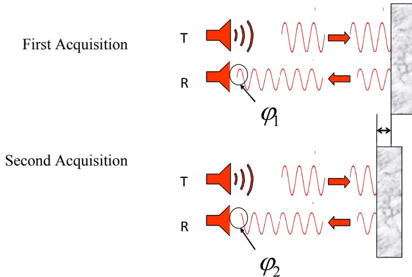
**Figure 3:** Data collection process in the Interferometric process (Lee 2010)
