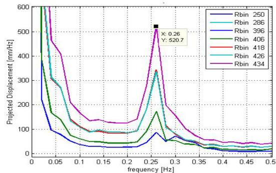
**Figure 6:** Soul Building frequency domain Data showing the structure natural frequency
