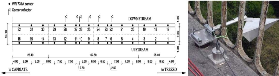
**Figure 8:** Location of accelerometers and passive targets on the central span (left), image of accelerometer and target installation (right) (Bernardini et al 2007)
