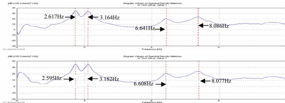
**Figure 11:** Frequency data measured using the accelerometers (top) and Interferometer (bottom) (Bernardini et al 2007)
