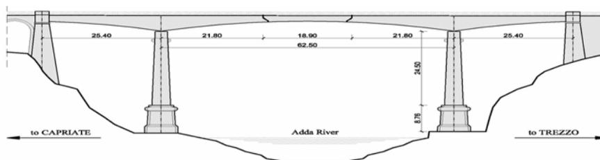
**Figure 7:** Schematic of the Adda River Bridge, showing the central span in question (Bernardini et al 2007)
