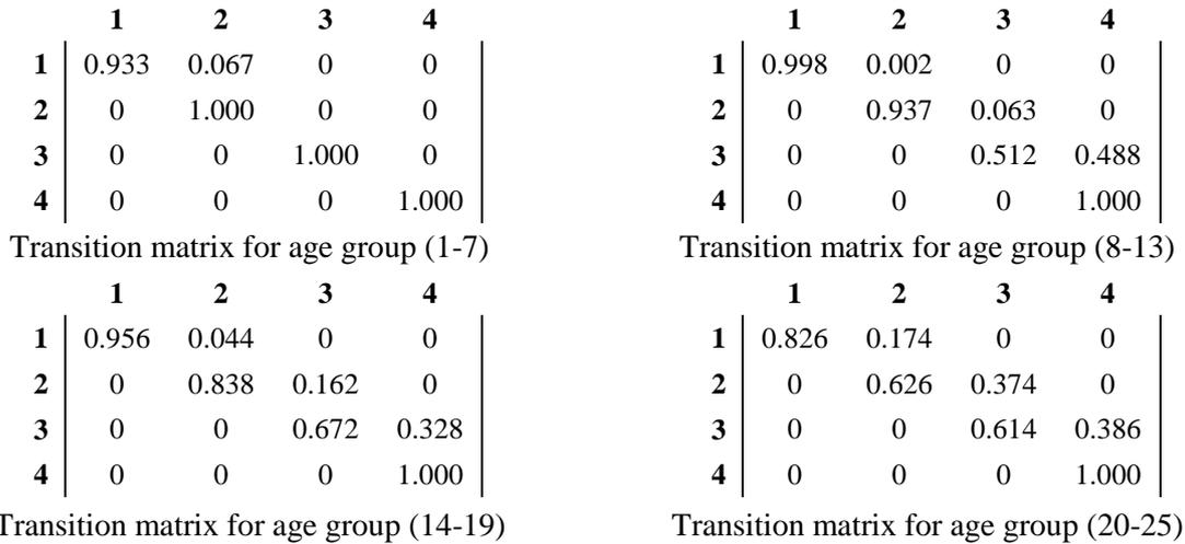
**Figure 6.** Transition probability matrices for bridge element type 4C
