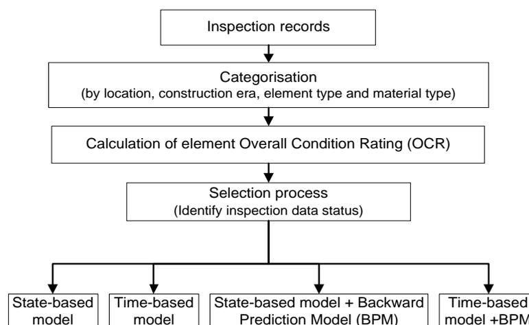
**Figure 1.** The components and procedures of the proposed integrated method
