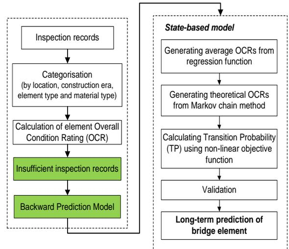
Figure 3. Procedure of the state-based model
