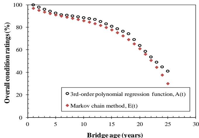
**Figure 7.** Comparison between the average  $A(t)$  from the 3<sup>rd</sup>-order regression function and estimated  $E(t)$  from the Markov chain method
