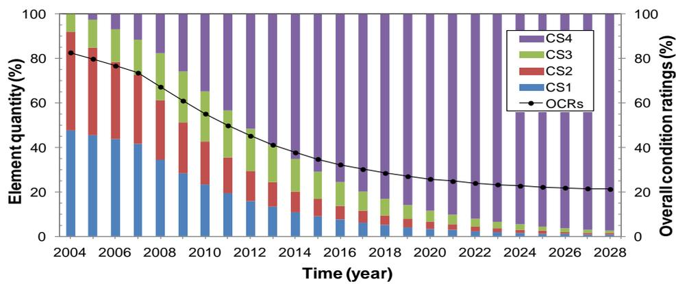
**Figure 8.** Long-term prediction for Bridge#XX54XX-element type 4C
