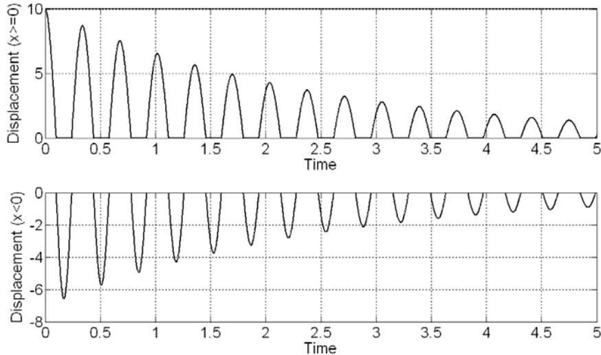
**Figure 3.** Separation of global responses into two parts at the stiffness interface ( $displacement=0$ )
