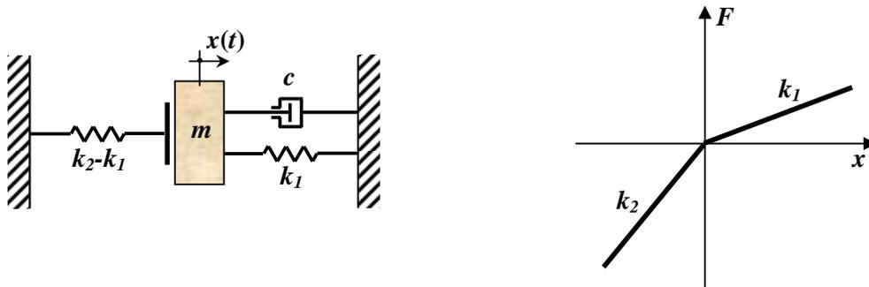
(a) physical model of a bilinear oscillator (b) restoring force model of the bilinear oscillator
