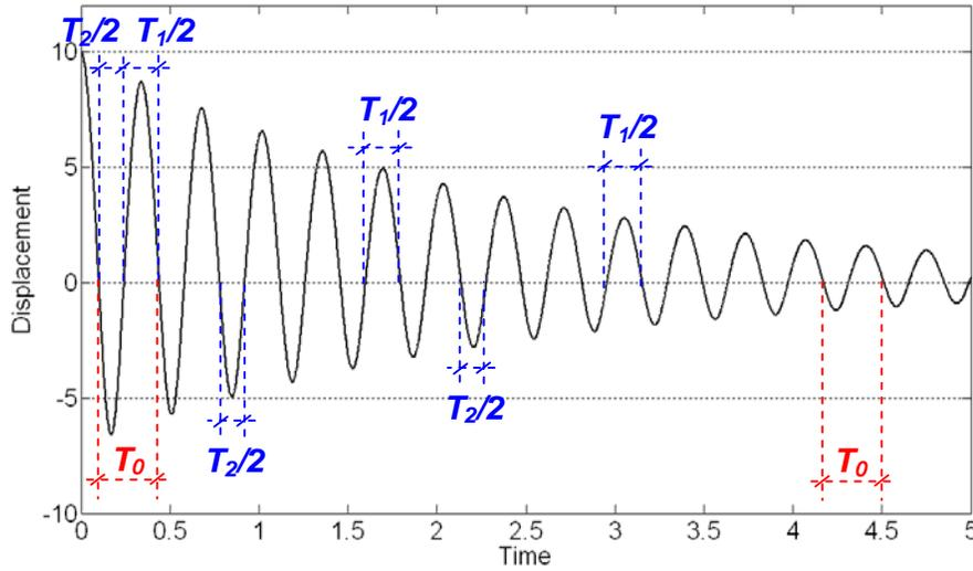
Note:  $T_1$  and  $T_2$  represent the oscillation periods corresponding to the two regions, respectively
