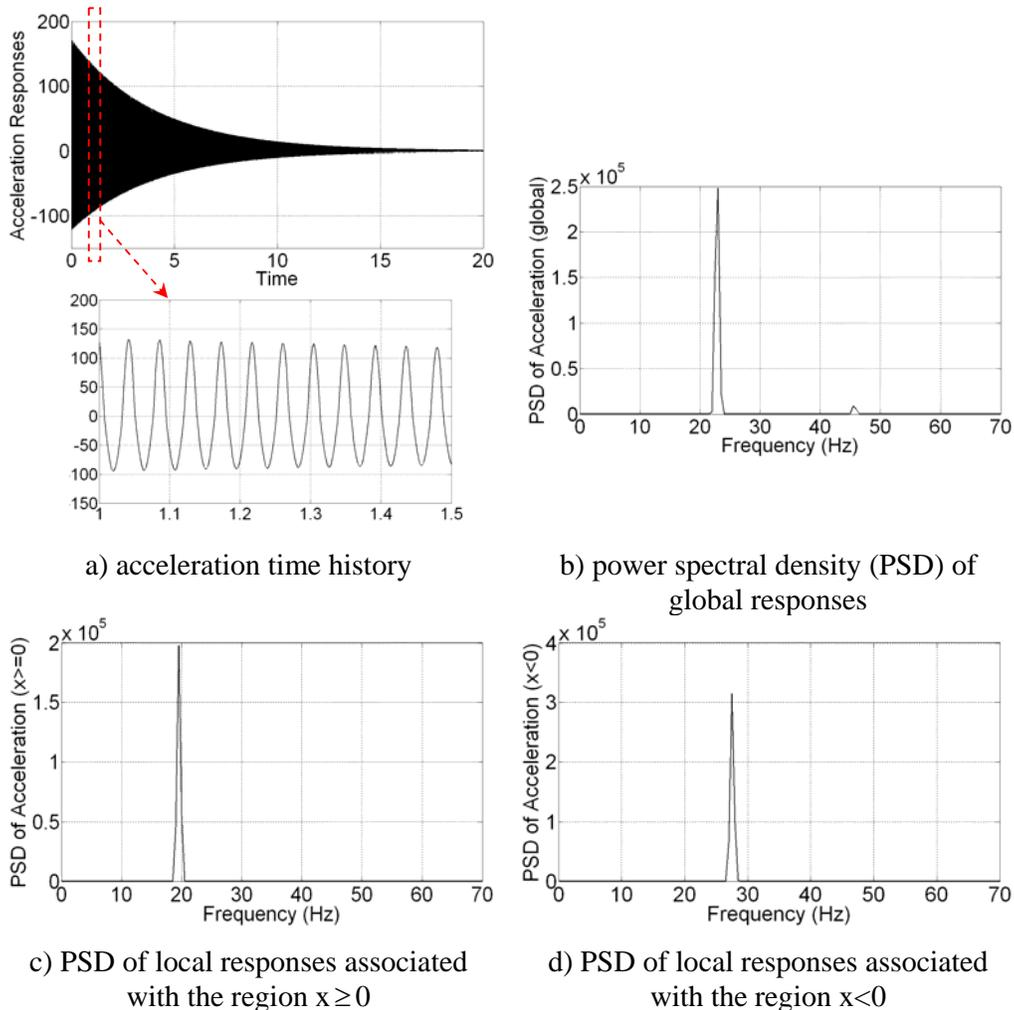
**Figure 5.** Acceleration responses and auto power spectral density of global and local response data
