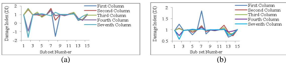
**Figure 4** Damage patterns obtained from the first floor when first, second, third, fourth and seventh columns are damaged with (a) 55% and (b) 10% damage severity
