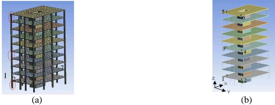
**Figure 1** (a) Damaged elements at first floor (b) FRFs measurement locations (Measurement points ‘7’, ‘8’, ‘9’, ‘10’, ‘11’ and ‘12’ are at mirror image of measurement points ‘1’, ‘2’, ‘3’, ‘4’, ‘5’ and ‘6’ respectively)
