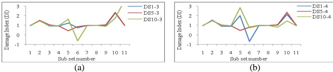
**Figure 2** Damage patterns from measurement point 2 subdivided by damage severity (a) 40% and (b) 55%
