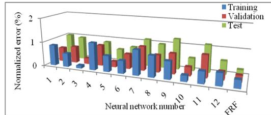
**Figure 3** Performance of networks trained with Damage Index (DI) values to identify damaged floor
