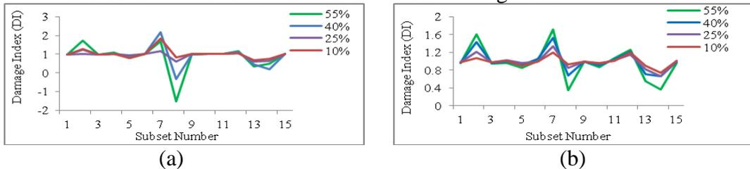
**Figure.5** Damage Index values from measurement point '1' for different severities when damage is at (a) column '1' and (b) column '2'
