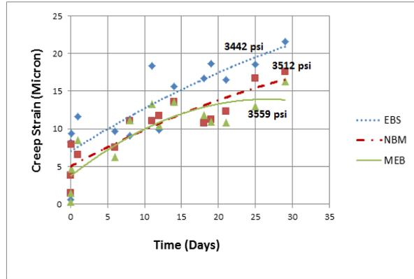
**Figure 2:** Effect of Compressive Strength
