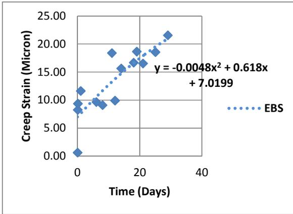
**Figure 4:** Equation of Creep Strain for Sample “EBS”
