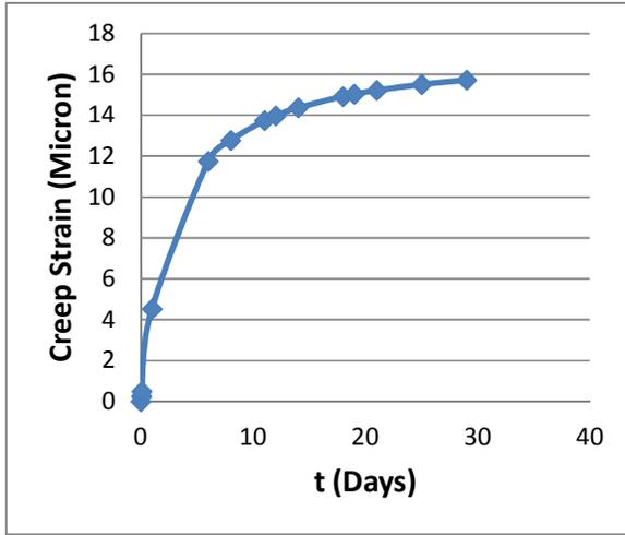
**Figure 8:** Theoretical values of creep strain.
