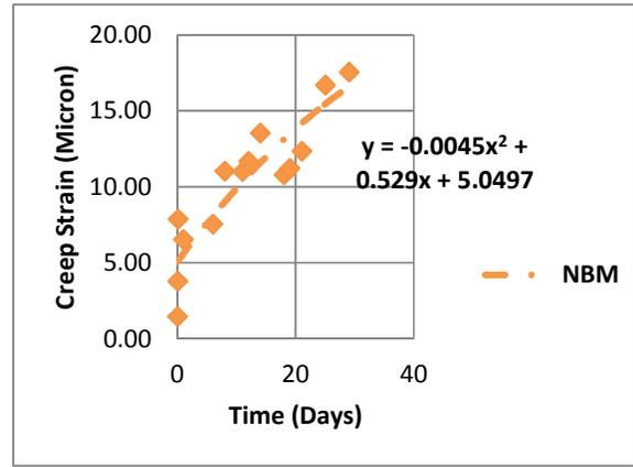
**Figure 5:** Equation of Creep Strain for Sample “NBM”
