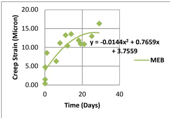
**Figure 6:** Equation of Creep Strain for Sample “MEB”
