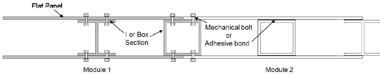
**Figure 1.** Proposed GFRP sandwich modular slab system assembled in the transverse direction
