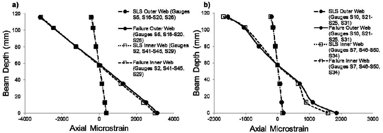
Figure 7. Axial strain distribution in cross-section at a) midspan and b) at span/6
