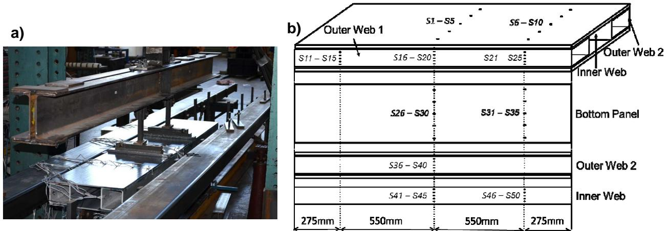
**Figure. 4a)** Experimental setup and **b)** strain gauge instrumentation
