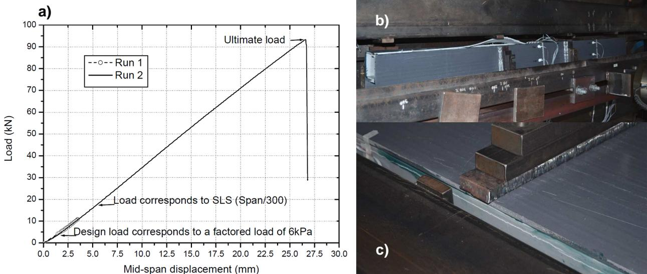
**Figure 5 a)** Load-displacement behaviour of sandwich beam at midspan; **b)** Shear failure at web-flange junction of one box section and **c)** of the other box section
