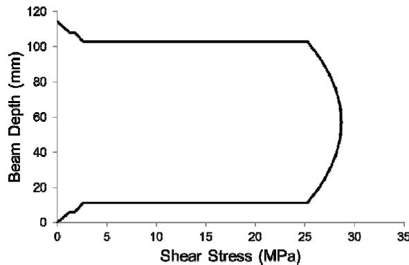
Figure 8. Shear stress distribution at failure load
