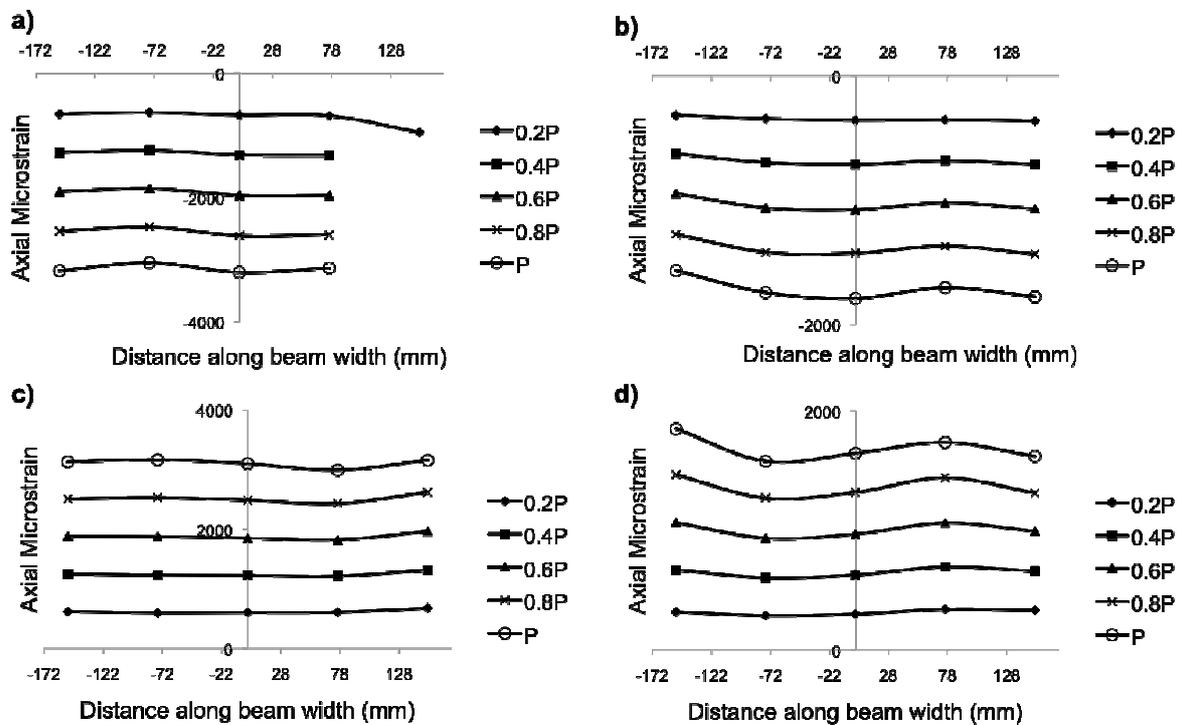
**Figure 6.** Axial strain distribution of **a)** the top facesheet at midspan (S1 to S5), **b)** the top facesheet at a distance span/6 from the support (S6 to S10), **c)** the bottom facesheet at midspan (S26 to S30) and **d)** the bottom facesheet at span/6 (S31 to S35).
