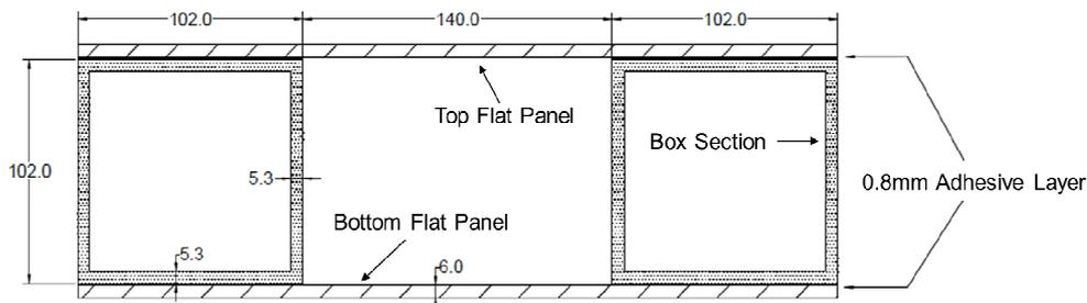
**Figure 2.** Dimensions of sandwich beam
