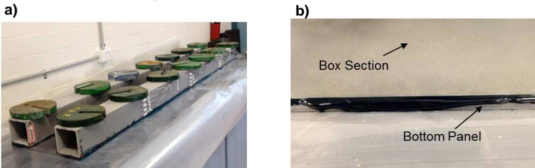
**Figure 3a)** Fabrication process of a sandwich beam with weights used to provide clamping pressure during curing of adhesive; **b)** Adhesive squeeze-out during bonding process
